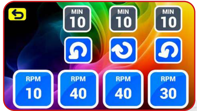
Set mixing speed, time and direction and quickly save and recall up to 6 different programs
